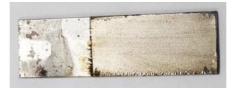
**Figure 10:** Photograph of a nickel layer deposited onto a mild steel substrate following electrolysis of ChCI: 2 EG containing 1.14 mol dm<sup>-3</sup> at 80 °C and current density of 1.5 A dm<sup>-3</sup> for 1 h. The substrate was etched in-situ by applying 1 A dm<sup>-2</sup> for 30 sec.
