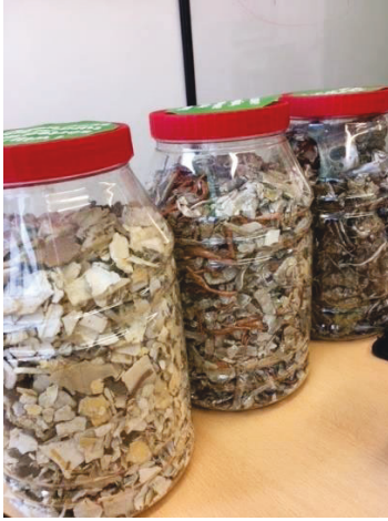
Plate 15 HIPS from a fridge reprocessing plant -site visit 2.
