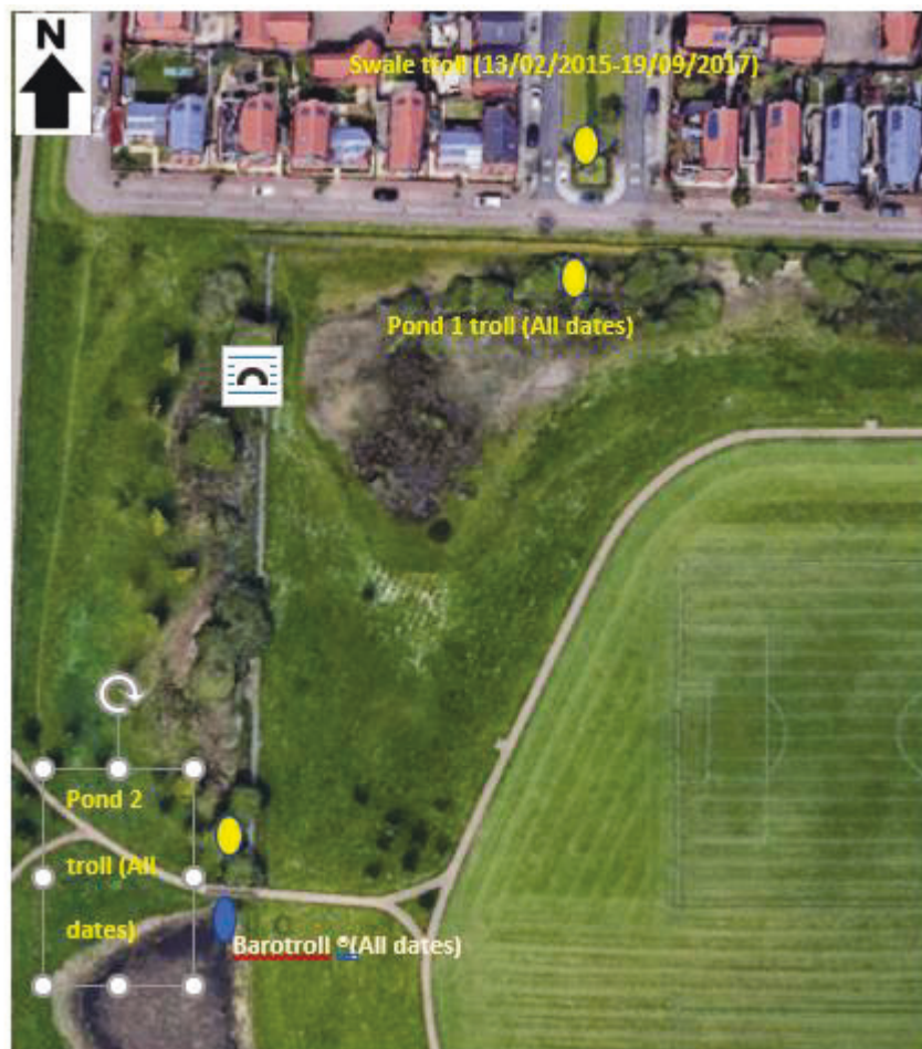
Figure 4.19: The position of all the trols (Rugged Trols in yellow; BaroTroll in blue) placed in the SUDS at Upton during May 2017(Google Earth, 2021e).
