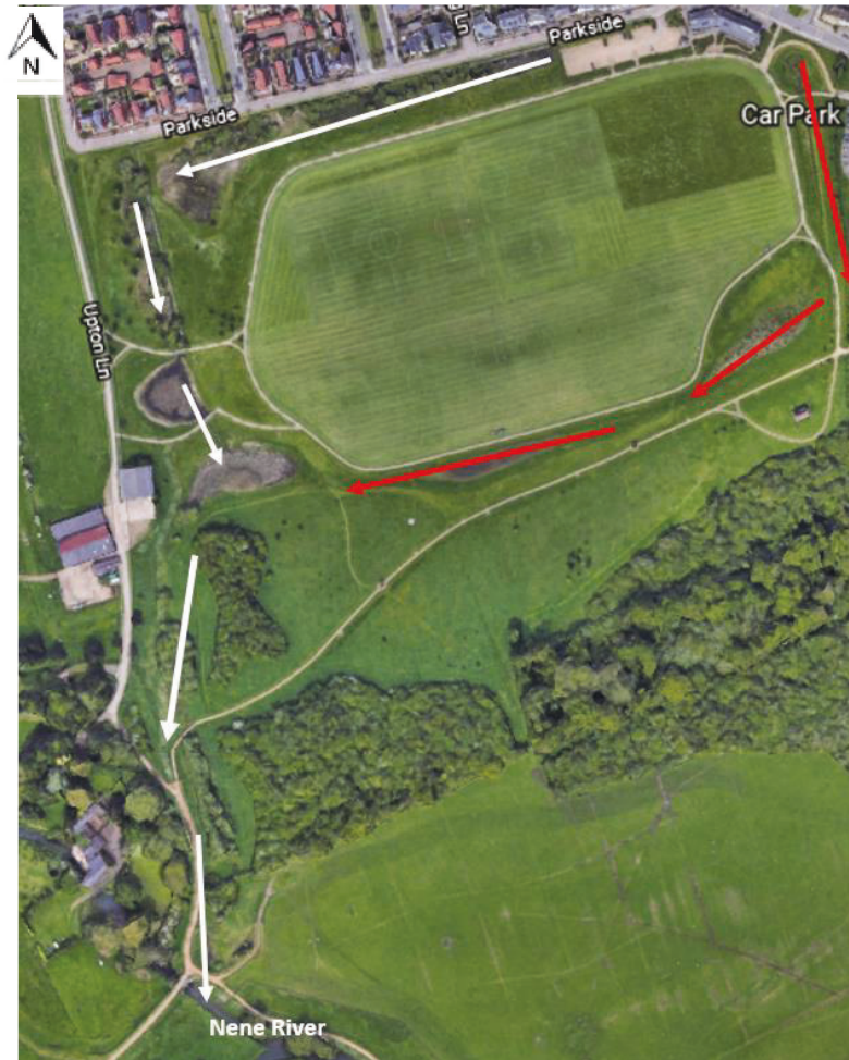
Figure 3.8: Representative diagram of the water movement round the site prior to discharging into the River Nene (Google Earth, 2021d).
