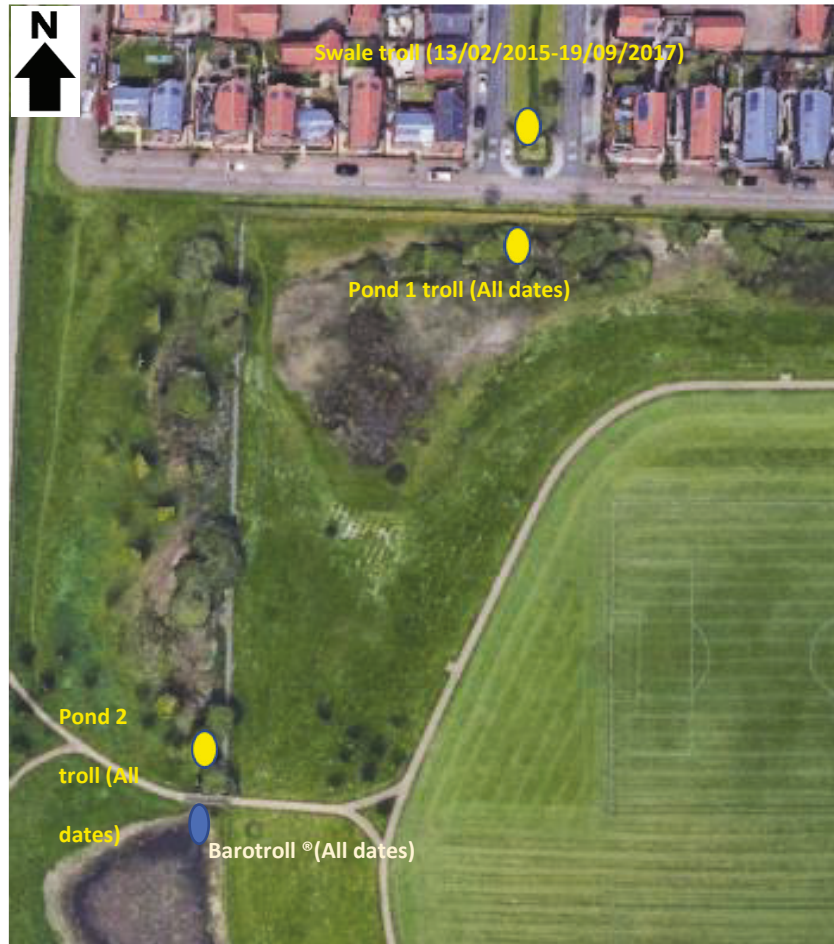
Figure 4.4: The position of all the Trolls® (Rugged Trolls® in yellow; BaroTroll® in blue) placed in the SUDS at Upton during the study period (Google Earth, 2021e).
