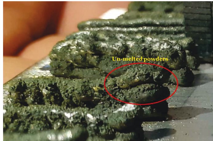
Figure 13 – Un-melted powders on the surface of the part.
