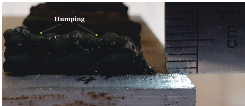
Figure 15- Humping phenomenon in part 4.
