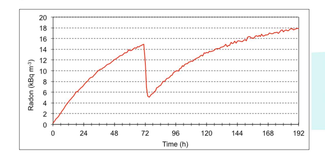
Fig 2. Radon Exponential Increase. Newmark Wrist Watch
