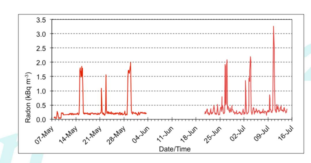
Fig 3. Radon Concentration in Room, May-July 2001.
