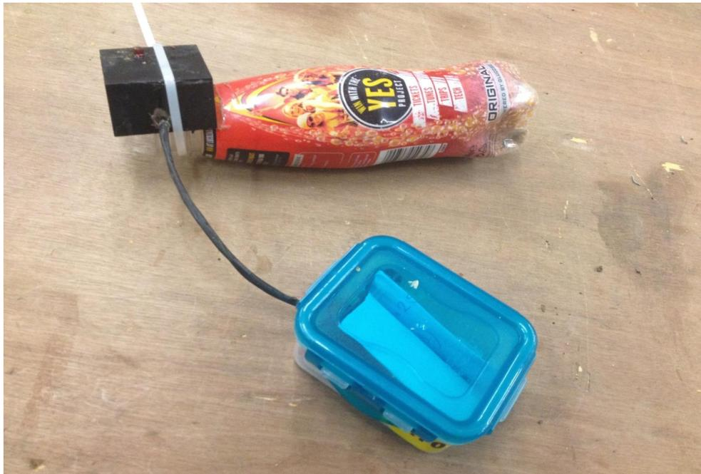
Figure 2.8 – Version 0.1 of the RFID trap. The reader is situated above the entrance of the bottle, the reader components were housed in the plastic water tight box. Traps were baited with Johnson and Jeff Cockatiel mix to encourage usage.
