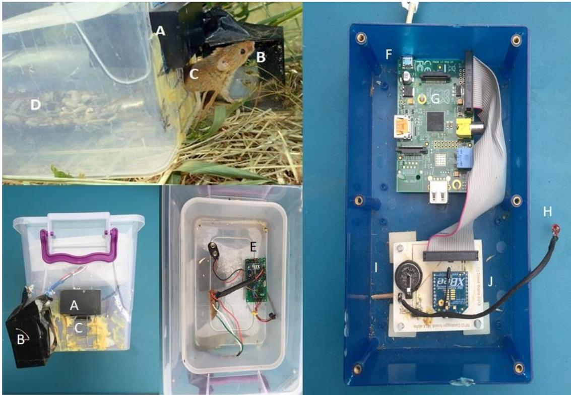
Figure 2.9 - RFID trap with *M. minutus* exiting, RFID trap and data logger. Components include: electronic reader (A), PIR motion sensor (B), trap entrance (C) and baited plastic drinks bottle (D), RFID trap printed circuit board components, this view shows the top of the trap, not accessible to the occupants (E), data logger (F), Raspberry Pi (model A) ® (G), LED data transmission indicator (H), real time clock (I) and Master Xbee radio (J) - (*M. minutus* picture courtesy of Upton (2015c)).
