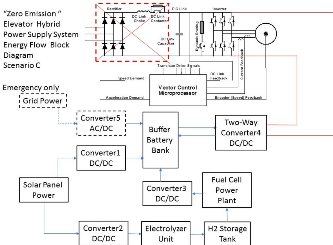
**Figure 7 Energy Flow Block Diagram – Scenario C**
