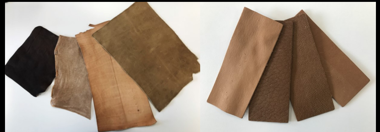
Black Tea Extract Rapeseed Meal Coffee Extract (main tan) Coffee Extract (Retan) Malt Grain Extract Rapeseed Meal Coffee Extract
